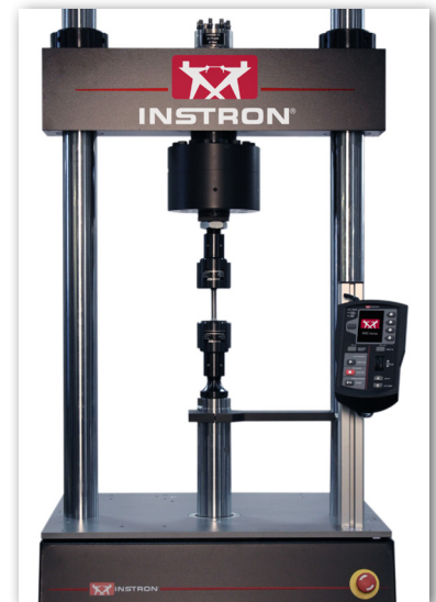
300 kN Split Tensile Holders for Testing .505 Button Head Specimens on 300LX
